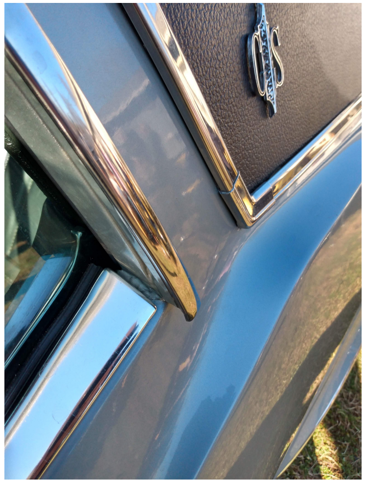
Close up detail showing vinyl top trim, roof drip rail trim and the B85 window sill trim.
